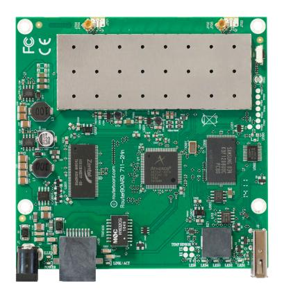
The RB711G-5HnD is a small 5GHz wireless router, it has built in wireless with **two chains**, a USB port and PoE/ Jack powering support. <u>Output power up to 25dBm!</u>
